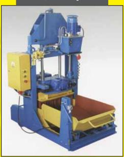
The HK-6 BIS is a small semi automatic block making plant, capacity 1,500 blocks per 8 hour day.
